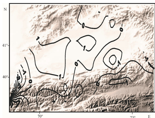
Figure 6. The velocity of vertical displacement (cm/year) in the territory of the Ferghana Depression. East longitude and north latitude in degrees.
